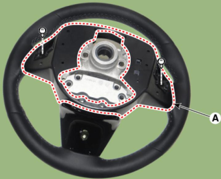
8. Disconnect the steering wheel remote control connector (A).
