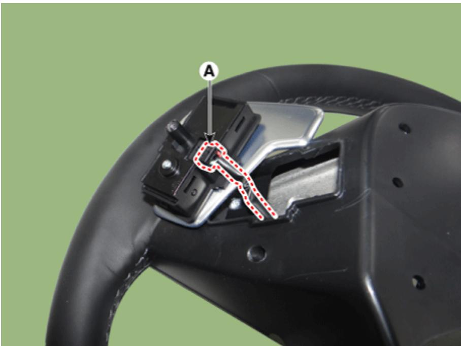
5. Remove the steering front cover (A) after loosening the mounting screws.
