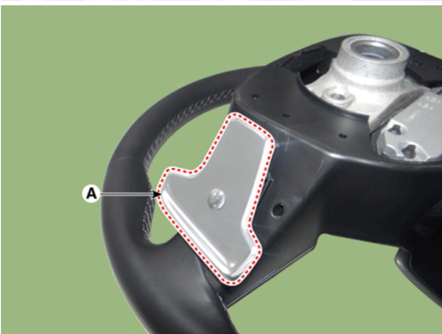
4. Disconnect the paddle shift switch connector (A).
